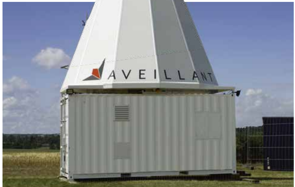
The Aveillant Theia holographic radar is a 3D sequential-scan unit that acquires continuous detail about every object, including all fine-motion detail in the Doppler spectrum.
